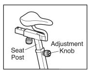
the seat post, and firmly tighten the adjustment knob. Make sure that the adjustment knob is engaged in an adjustment hole.
