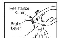
To stop the flywheel, push the brake lever downward. The flywheel should quickly come to a complete stop.
